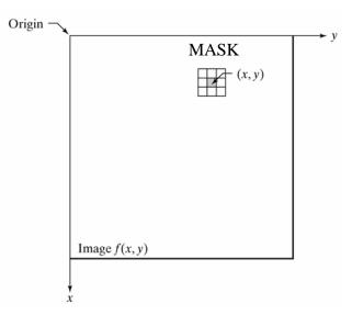
and translated across all possible pixel positions on the image. A new (filtered) image is produced by replacing the intensity value at the center by a linear combination of the intensity values of the center pixel and all neighboring pixels covered by the mask. The coefficients (a-i) in the mask array give the weights of each pixel in the linear combination. Here is an example:
