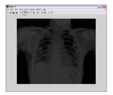
Note that in the figure toolbar we have buttons that allow us to zoom parts of the image. The syntax **imshow(f, [low high])** displays all pixels with values less than or equal to **low** as black, all pixels with values greater or equal to high as white. Try
