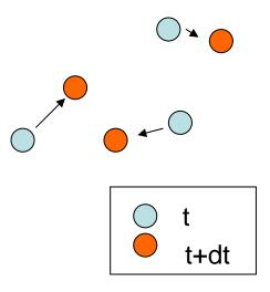
It is often the case in image acquisition that the time interval between successive frames is so small that these moving particles move only small distances during this time interval. In such a case, it is often adequate to match particles with the closest ones nearby. In such a case, we find a matching that minimizes a cost function determined by the distance traveled by particles. A cost function that works well for diffusive motion is given by the sum of squares of the distances:
