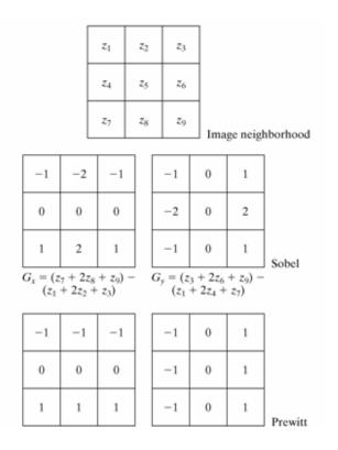
The Prewitt and Sobel operators are among the most used in practice for computing digital gradients. The Prewitt masks are simpler to implement than the Sobel masks, but the latter have slightly superior noise-suppression characteristics.
