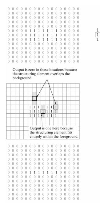
In the following example one can see how different erosions affect the features of an image
