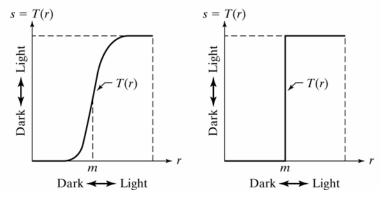
In the limiting case of E >> 1, the image is thresholded at the intensity **m**. Try the following commands
