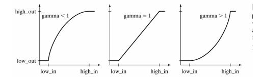
Here **low\_in** and **low\_high** give the low and high grayscale intensity values for the contrast adjustment, and **gamma** gives the exponent for the transfer function.
